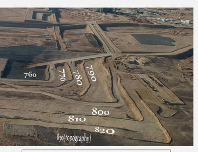
Figure (1): mine benches and it levels
