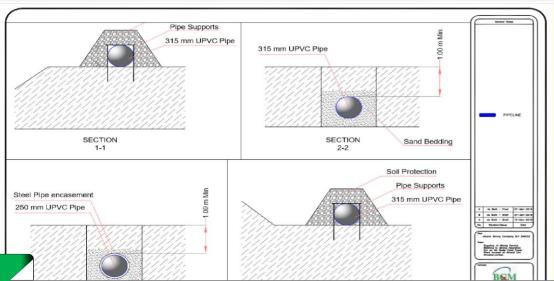
Ash Spreader Assembly Pads and surface water drainage system Design drawings
